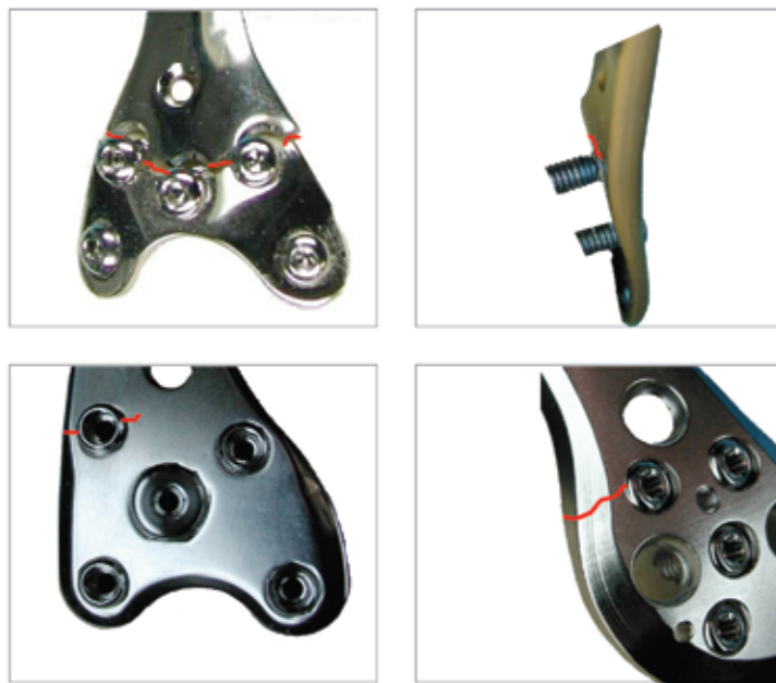
Figure 6: Failed Specimens from l. to r. DCP™ Condylar Buttress Plate, LISS™, LCP™ and AxSOS™.
