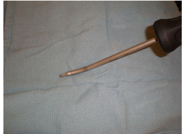
Figure 4. A flexible screwdriver with jigsaw segmentation.
