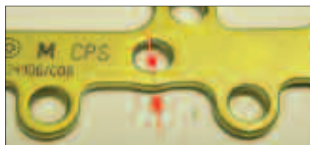
Figure 11: Failure pattern of Darco® CPS plate, medium, 3 point bending, (no figure of VariAx plate since no fracture occurs)
