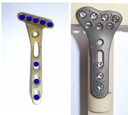
Figure 5: left: Screw positions of the Synthes® LCP plate (marked with blue dots), right: Screw positions of the Stryker® VariAx plate
